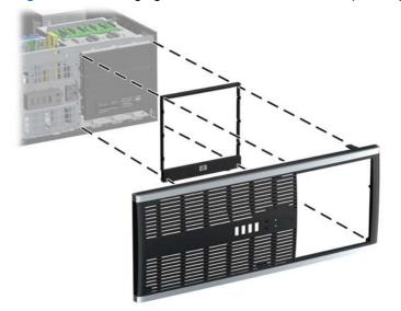
Figure 5-59 Changing from a Minitower to a Desktop Configuration
